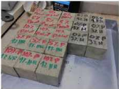
The test specimens were stored in moist air for 24 hours. A minimum of 3 specimens should be tested at each selected age group.
