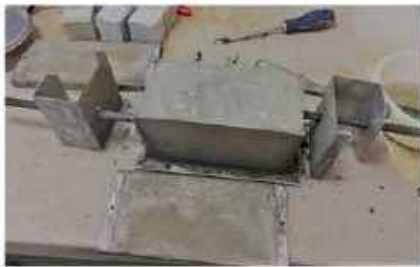
After 24 hours the samples are removed from the metal block
