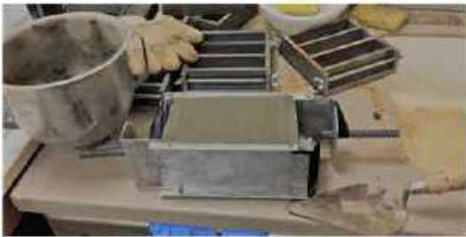
Fill the concrete in layers; compact each layer and level the top surface
